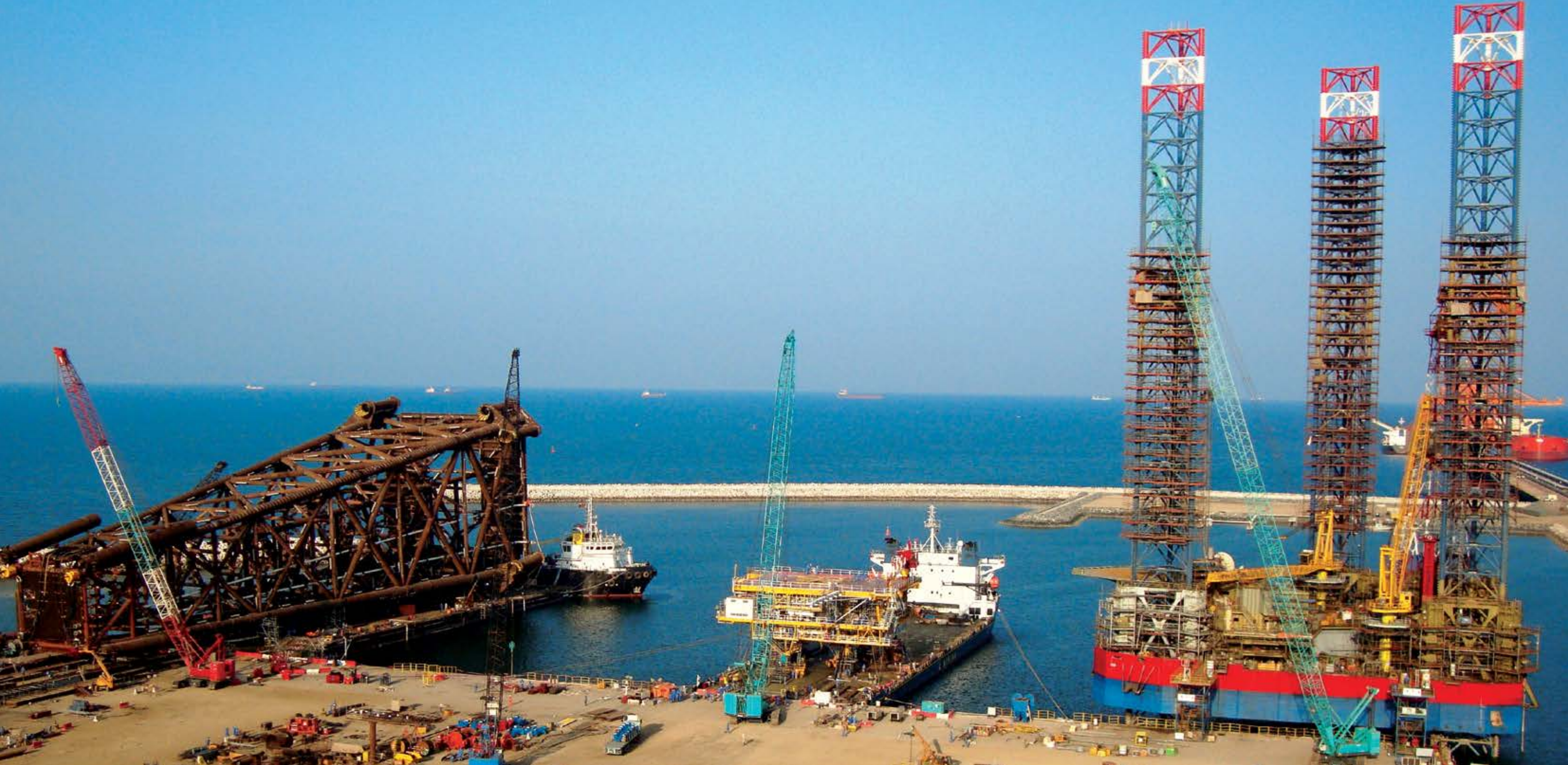
L&T's modular fabrication facility at Sohar in Oman has the capability to execute large scale fabrication up to 20,000 tonnes. Picture shows a jacket, a platform and a jack-up rig.
