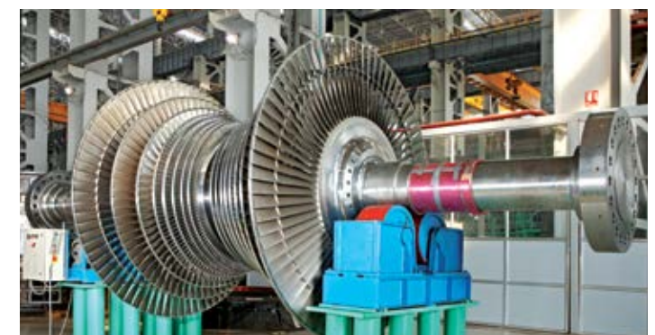
Supercritical turbine being assembled at L&T's Hazira Campus.
