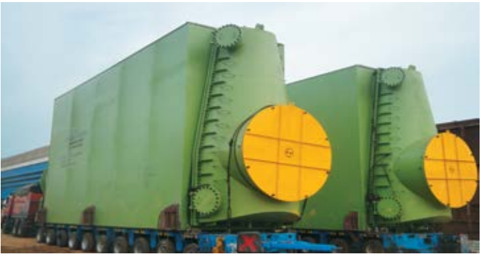
Surface condensers, each with more than 24,000 titanium tubes, are ready for transport to a 2 x 800 MW power plant at Krishnapatnam in South India.
