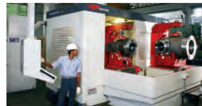
Five-axis machining centres ensure dimensional accuracy and consistency.
