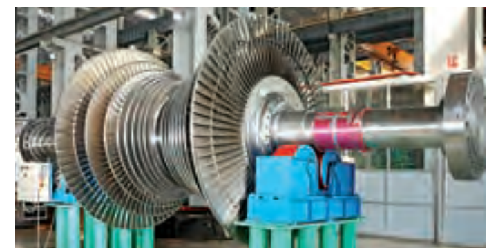
Supercritical turbine being assembled at Hazira Campus.
