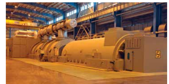
Enclosed turbine at a supercritical power project.
