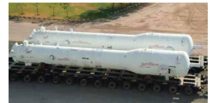
Steam generators for Pressurised Heavy Water Reactors.
