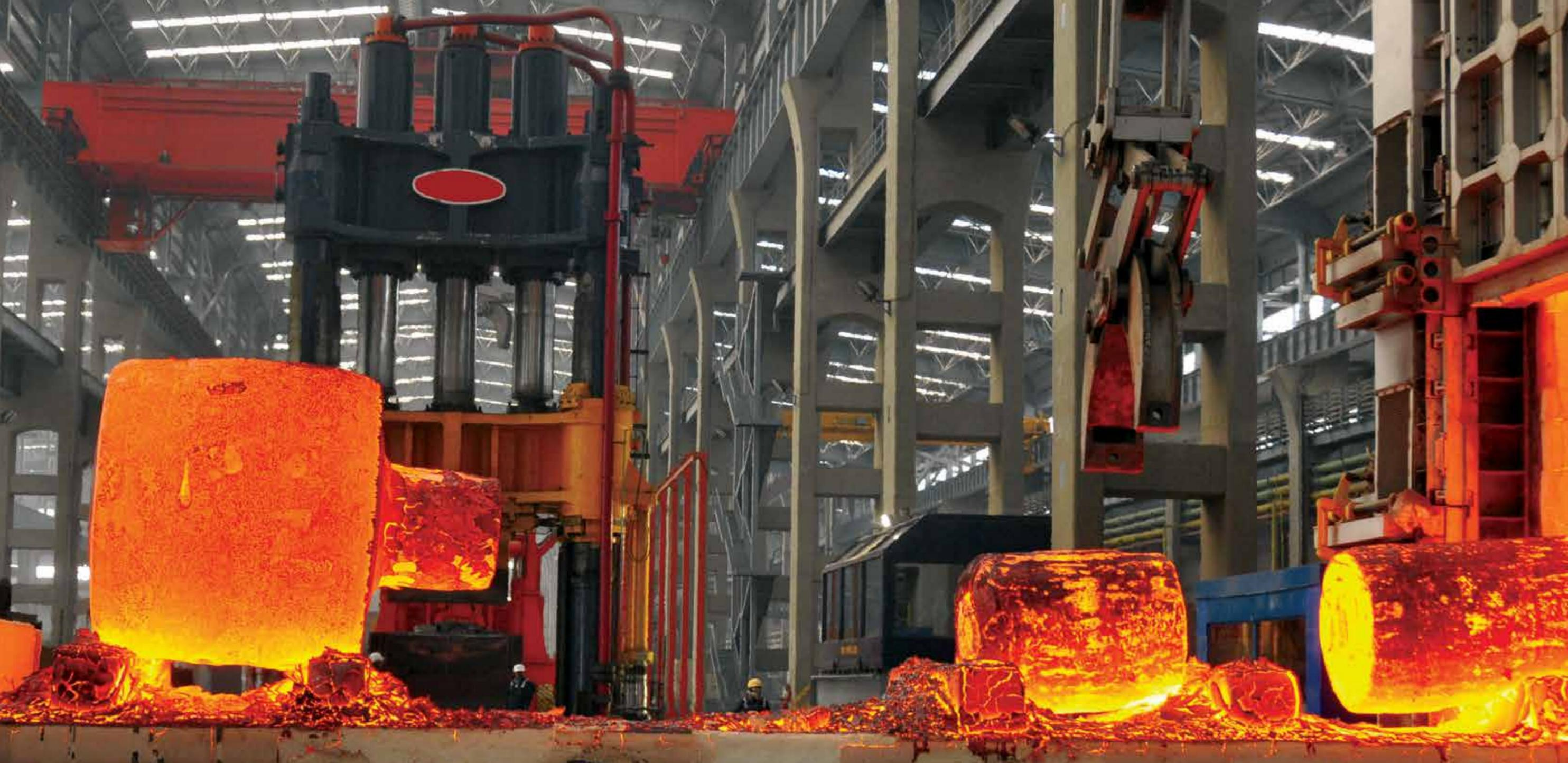
*L&T's nuclear-grade forge shop at Hazira (near Surat) – one of Asia's largest. It offers a wide range of finished forgings for the nuclear, hydrocarbon and power sectors, and can manufacture single-piece forgings of up to 120 MT.*
