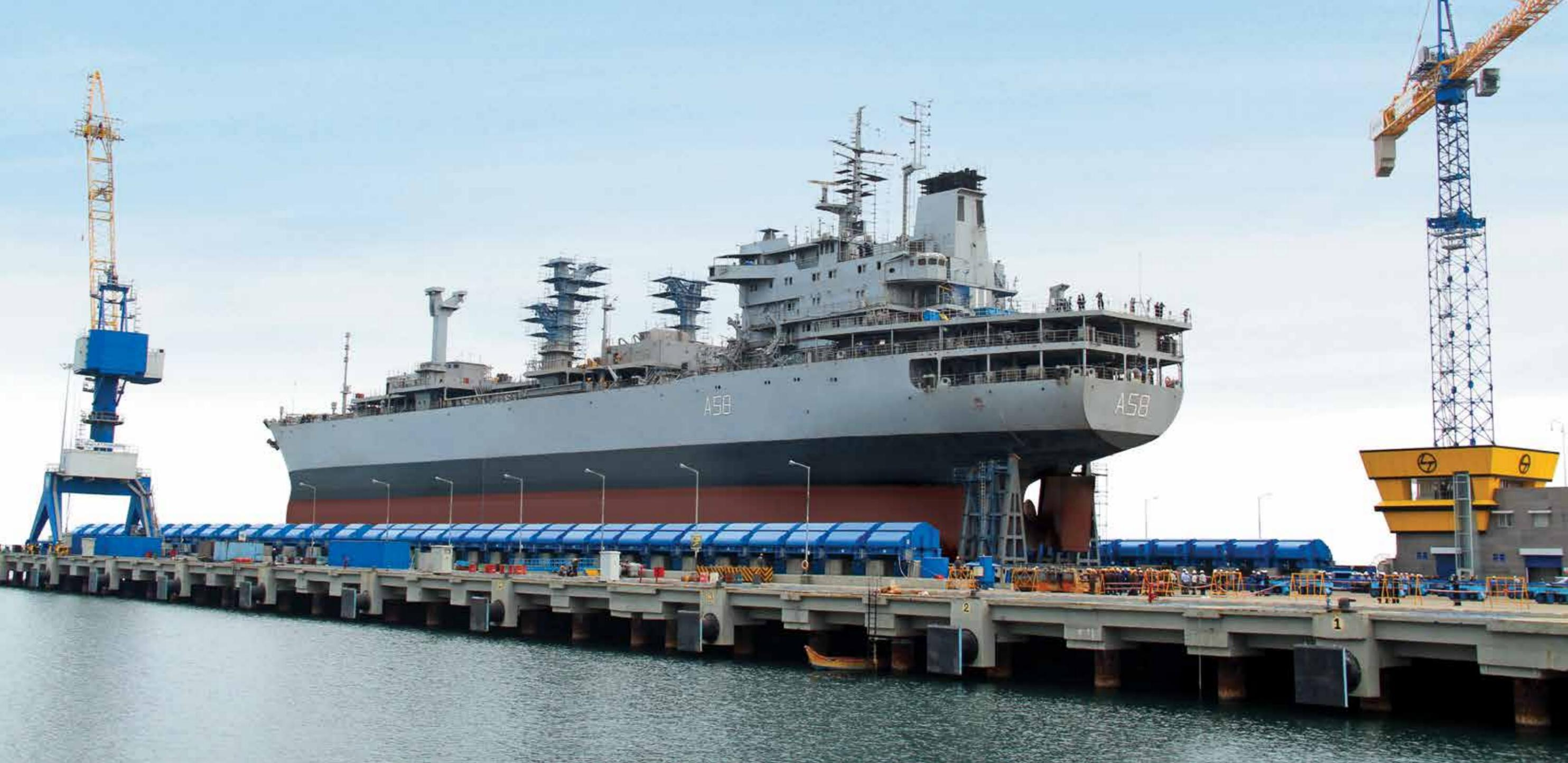
A 28,000 DWT defence vessel on the ship-lift at L&T's shipyard at Kattupalli. L&T undertakes ship design, building, maintenance and repair services for defence and commercial vessels.
