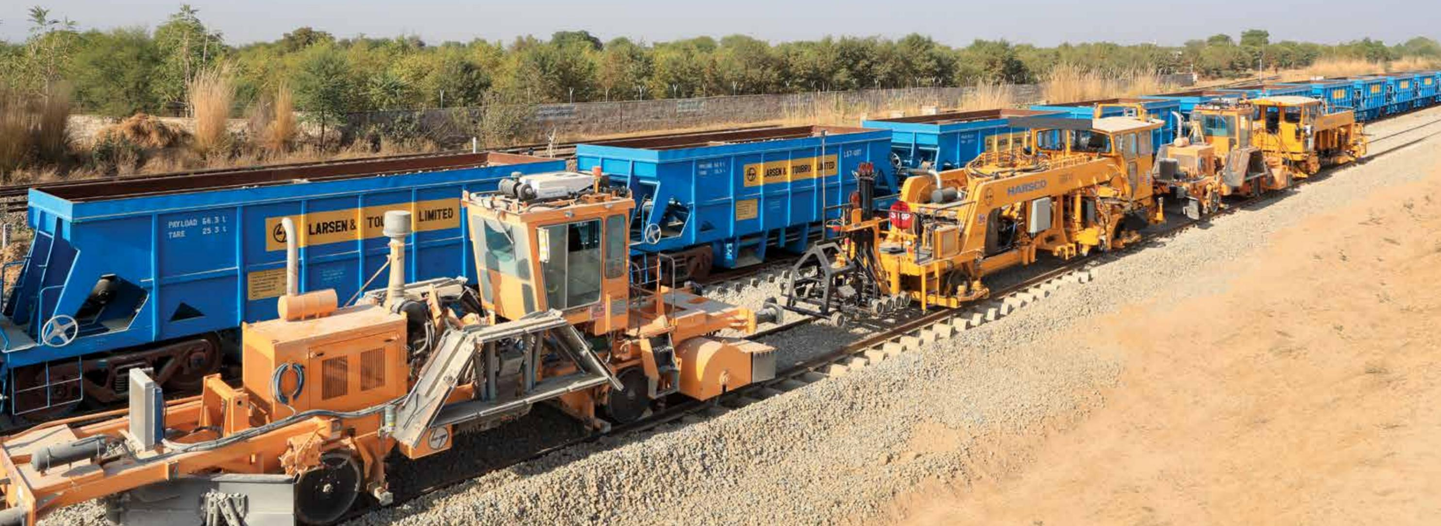
Capable of laying 2 km of tracks per day, the new track construction machine, owned by L&T, sets a benchmark in high-speed rail construction on the Western Dedicated Freight Corridor project. L&T is currently executing a number of prestigious railway projects in India and the GCC region.
