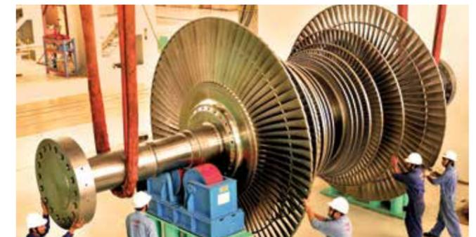
Supercritical turbine being assembled at L&T's Hazira Campus.
