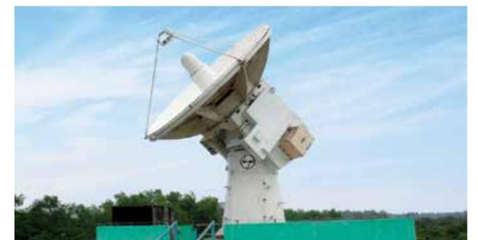
*Monopulse tracking radar – one of many indigenous radars and tracking systems developed by L&T.*
