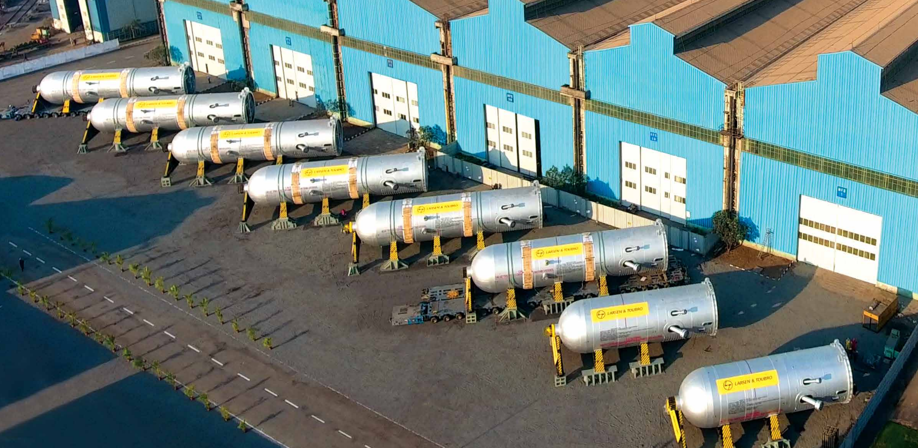
Eight ARDS reactors line up for despatch to the Refinery and Petrochemical Integrated Development (RAPID) Project of Petronas, Malaysia. Weighing a total of 7000 MT, these Cr-Mo-V reactors will help Petronas meet Malaysia's objective of establishing new areas of growth aimed at improving the quality of life.
