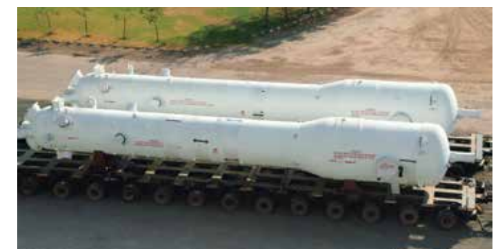
Steam generators for pressurised heavy water reactors. L&T is certified by ASME to use 'N' and 'NPT' stamps for the manufacture of equipment and systems.
