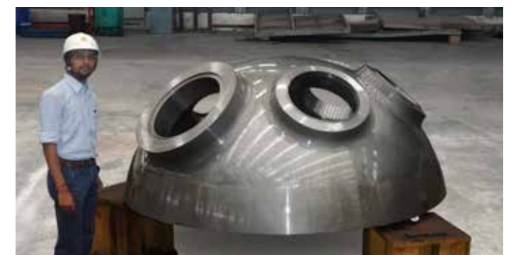
Dished ends forged at the Forging facility at Hazira, Gujarat.
