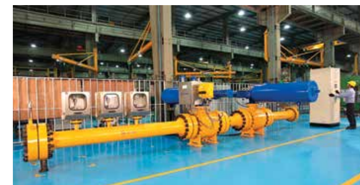
The first HIPPS (High Integrity Pressure Protection System) designed and manufactured in India. L&T Valves is a leader in safety instrumented systems for critical services in the energy sector.
