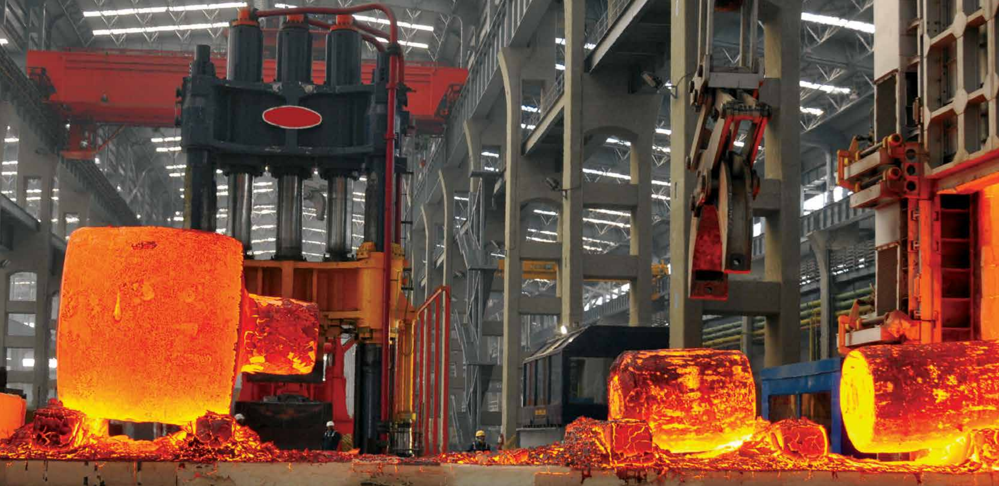
L&T's nuclear-grade forge shop at Hazira (near Surat) is one of Asia's largest. It offers a wide range of finished forgings for the nuclear, hydrocarbon and power sectors, and can manufacture single-piece forgings of up to 120 MT.
