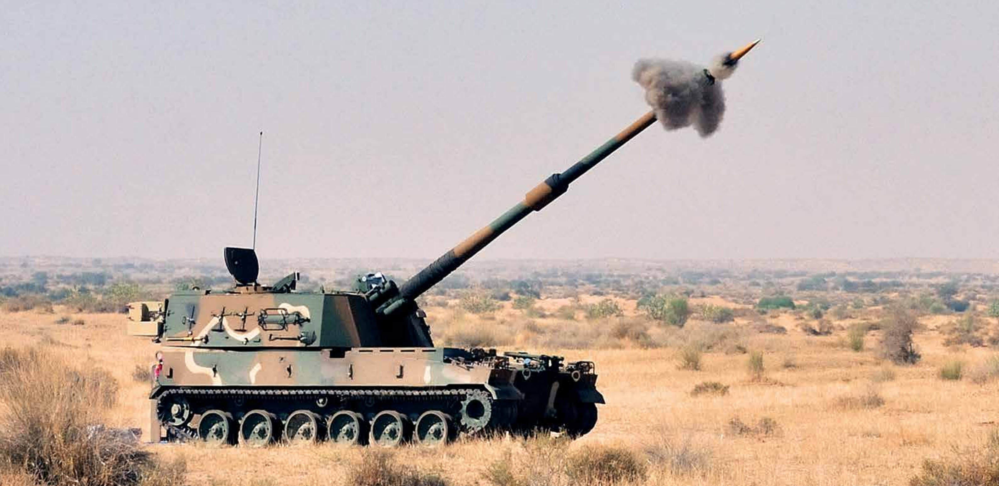
K9 Vajra-T 155mm/52 Cal Self-Propelled (SP) Tracked Gun is being built in collaboration with Hanwha Techwin. Designed for all terrains, it will give the Indian Armed Forces an advantage against border incursions.
