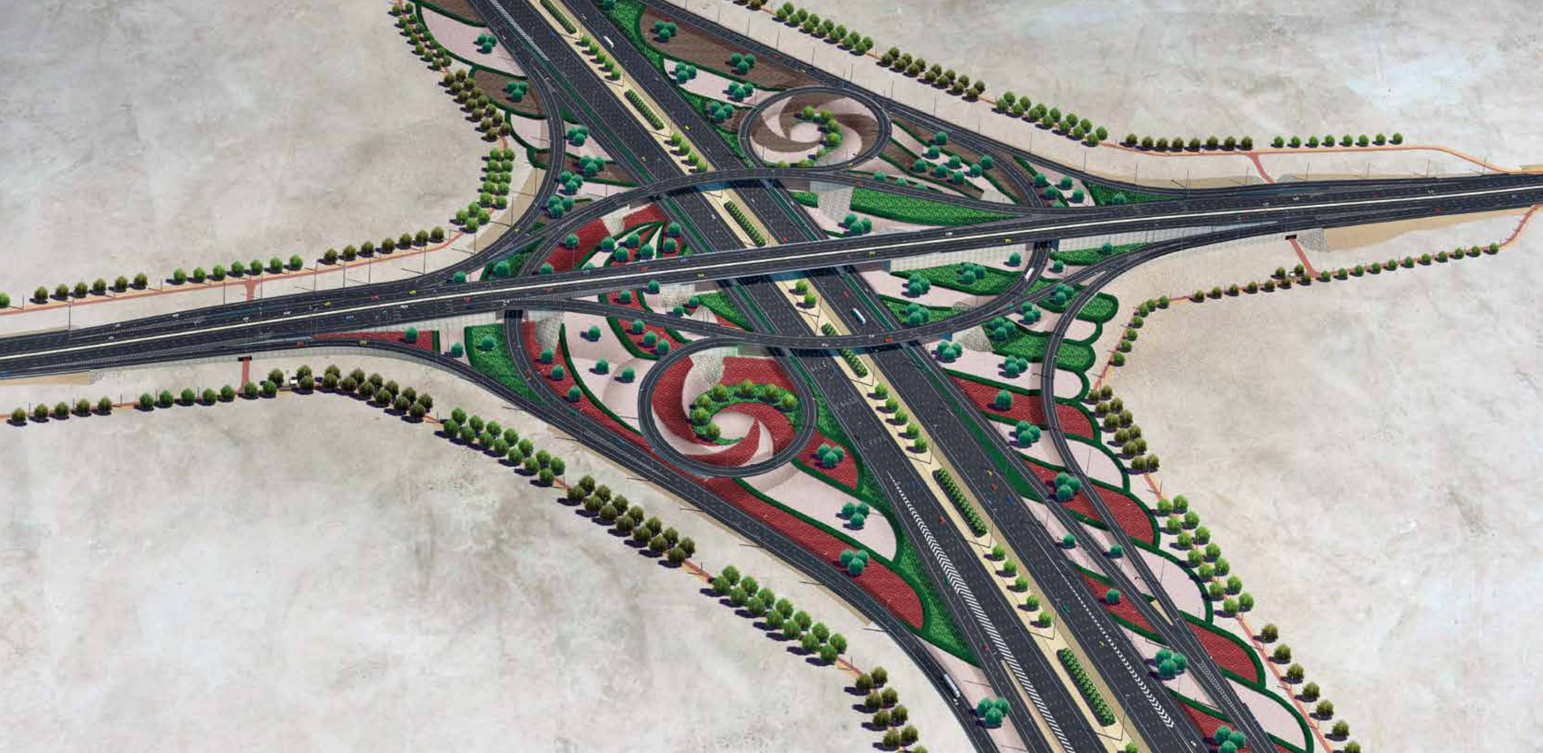
Artist's impression of the Al Wakrah Bypass Road in Qatar, consisting of five major interchanges including 20 bridges, three bicycle overpasses, eight vehicular underpasses, three pedestrian bridges and vehicular tunnels. This is one of L&T's many complex transport infrastructure projects in India and the GCC.
