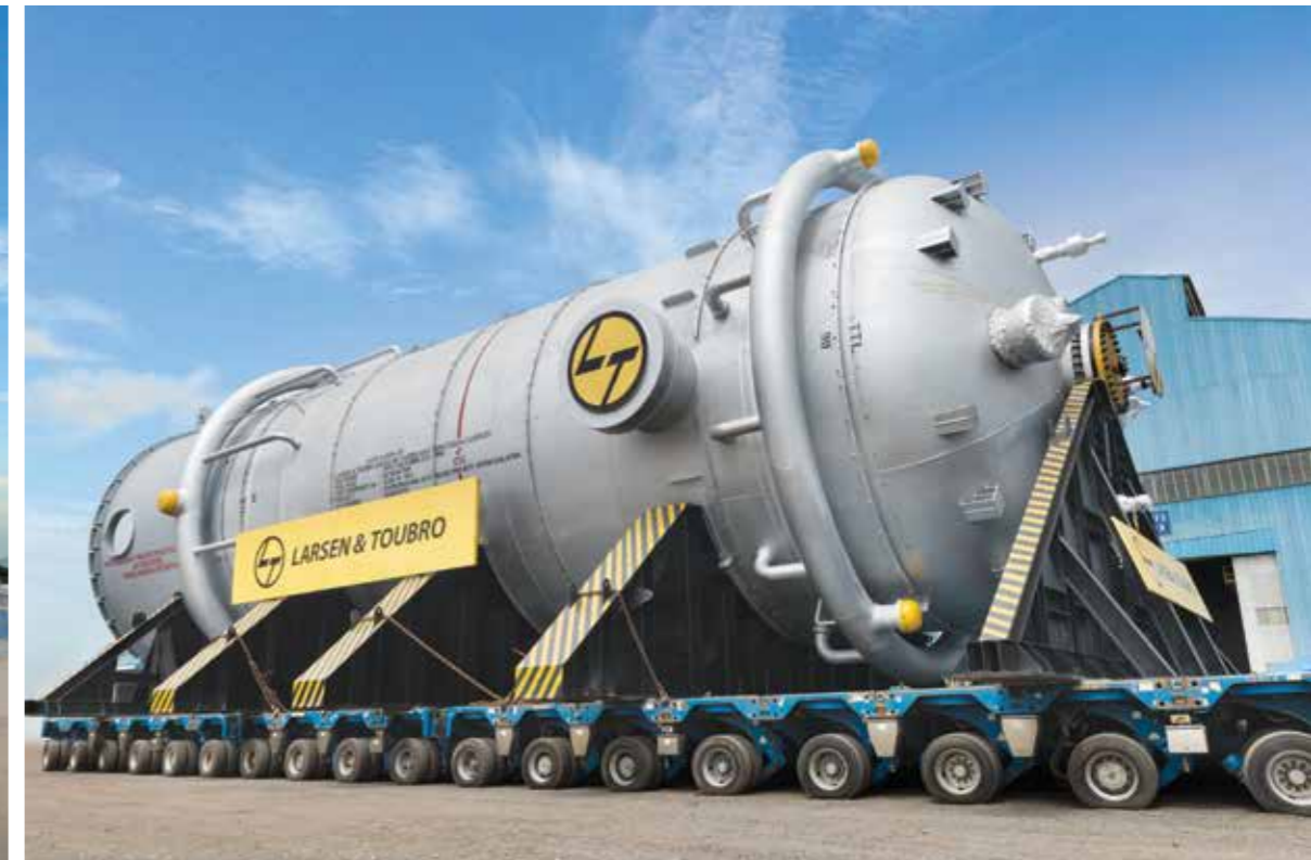
Ethylene Oxide Reactor
