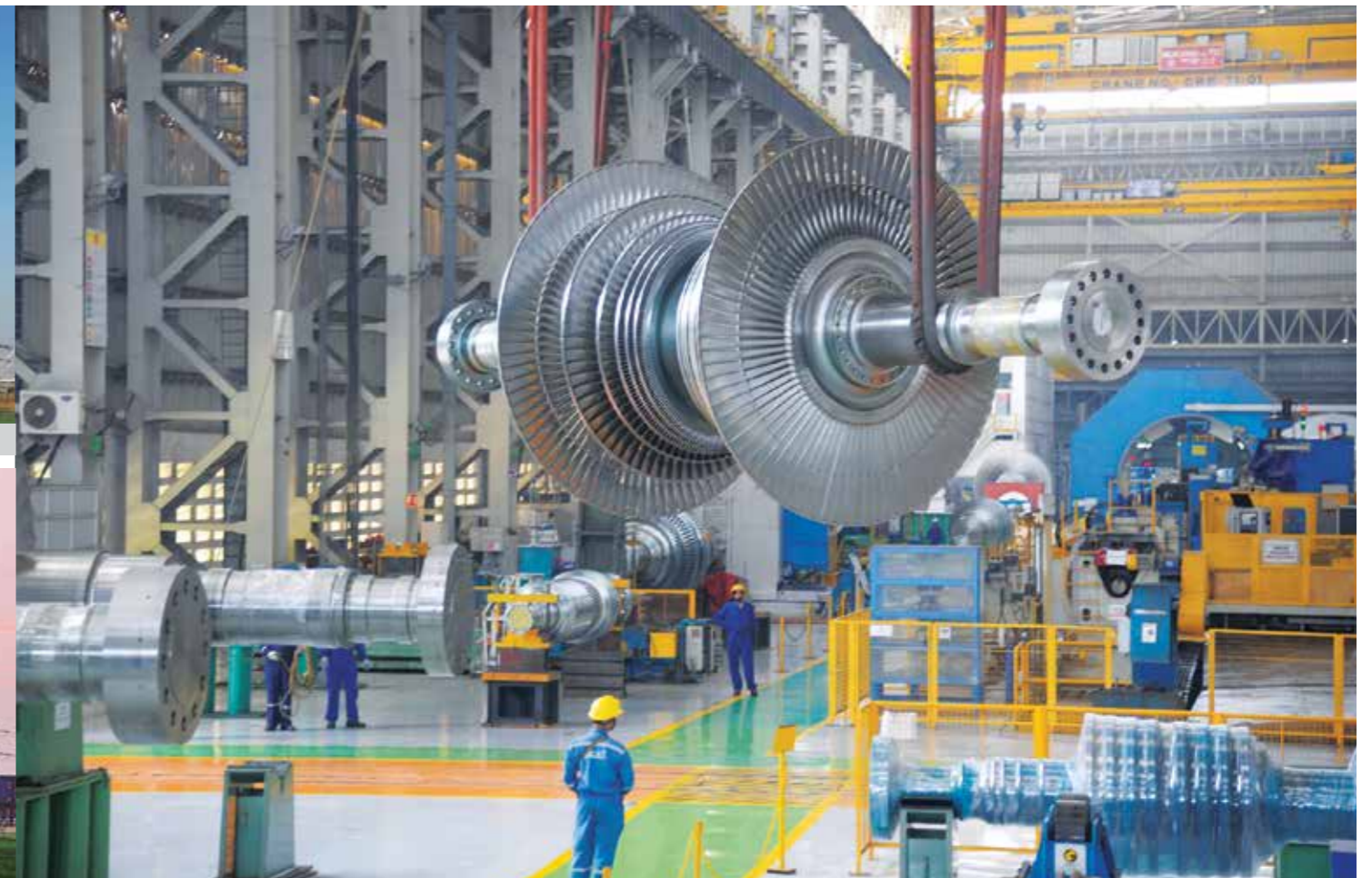
Supercritical turbine being manufactured at Hazira, Gujarat
