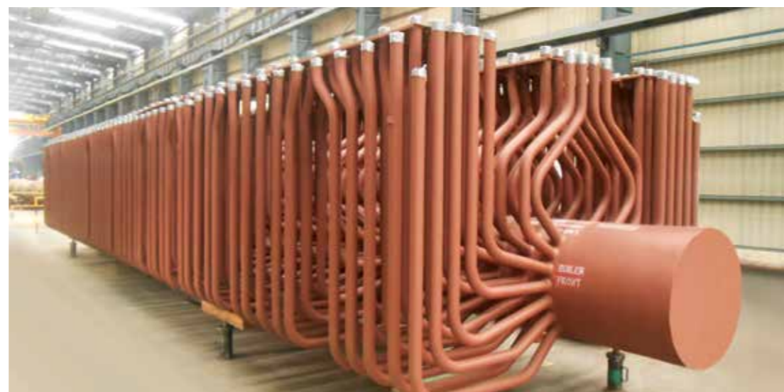
Boiler internals being manufactured at Hazira, Gujarat
