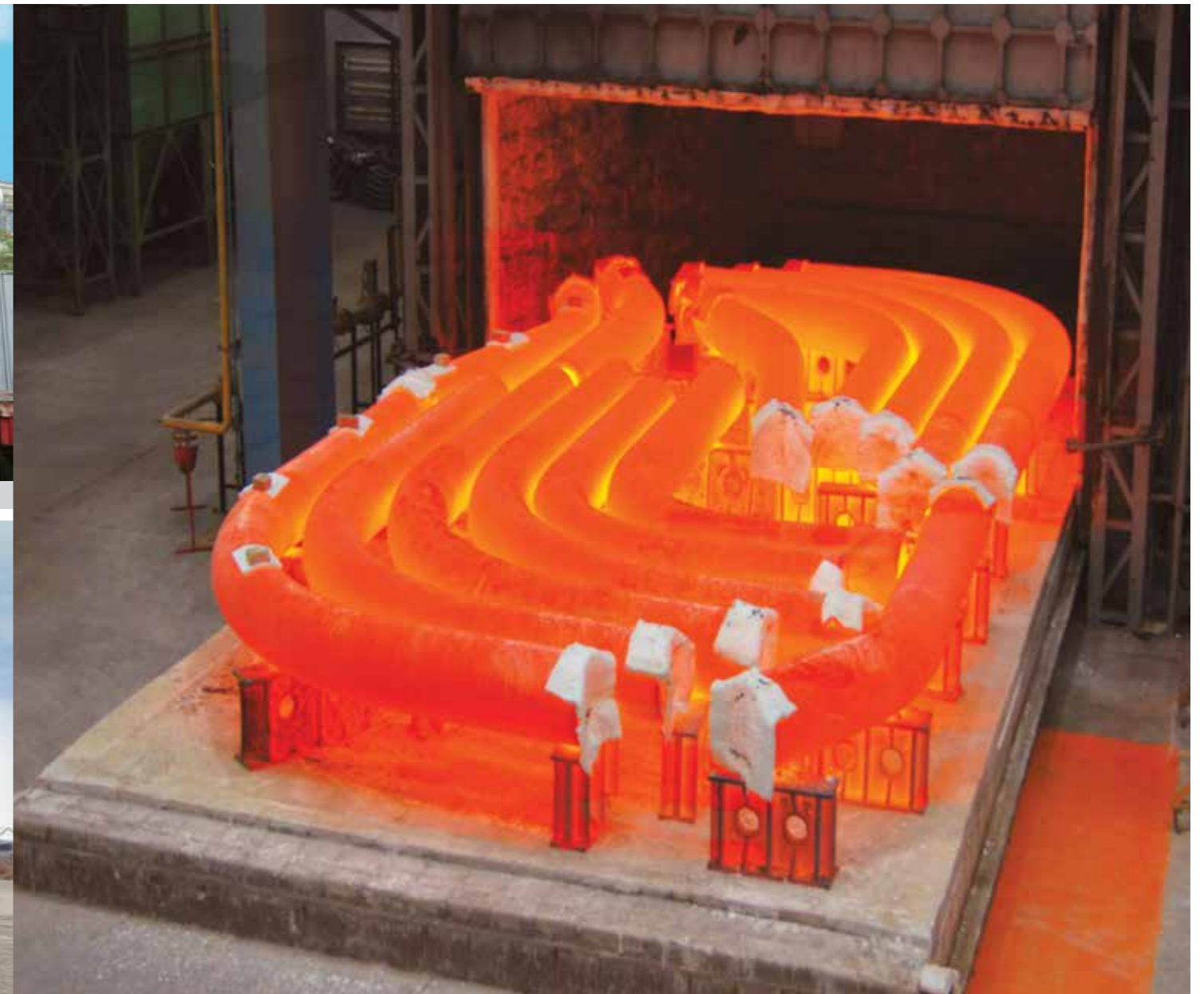
Critical Piping Spools undergoing heat treatment
