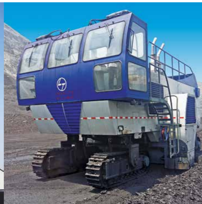
KSM-404 Largest Surface Miner in Indian Coal Mines at Gevra, Chhattisgarh - Manufactured by L&T at Kansbahal
