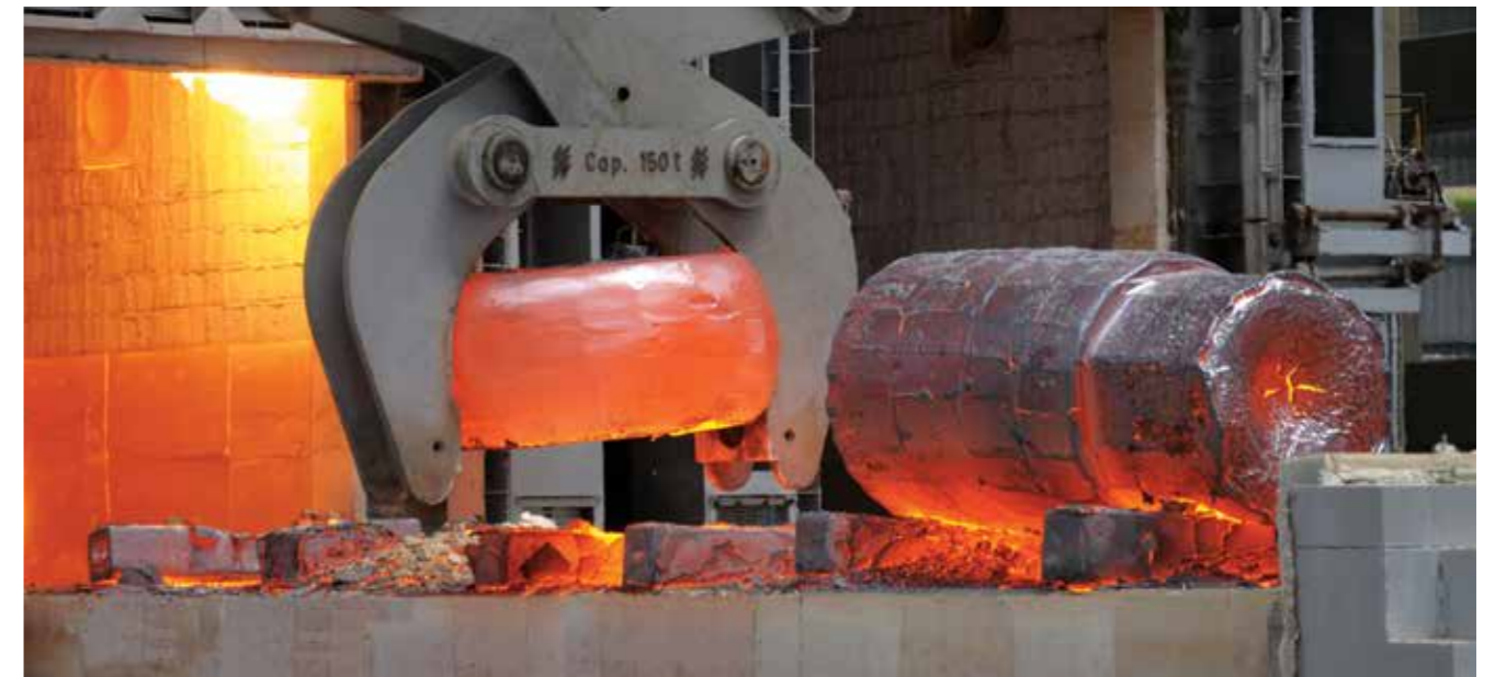
L&T's nuclear-grade forge shop at Hazira (near Surat) is one of Asia's largest. It offers a wide range of finished forgings for the nuclear, hydrocarbon and power sectors, and can manufacture single-piece forgings of up to 120 MT
