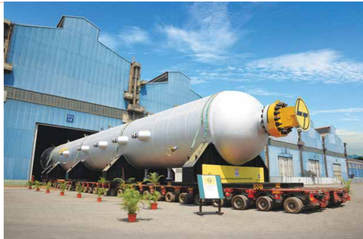
India's heaviest Hydrocracking Reactor (1858 MT)
